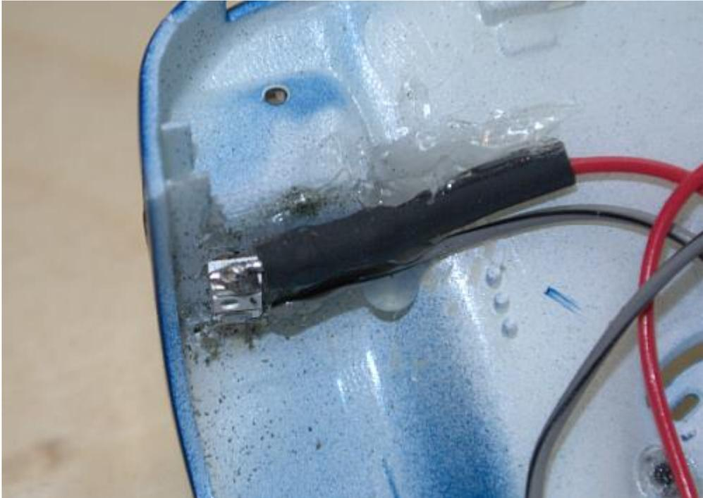
Figure 10. Shallow profile headlight LED mounted in Slot.it Porsche 962 IMSA.
